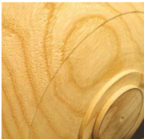
▲ Pic.10 Here's the difference between what he started with and the finish that can be achieved. Even though he is going to heavily texture the piece he does like to start off with a well-turned surface
